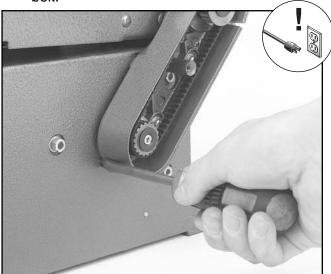
Figure 24. Tensioning the drive belt.
